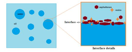
Figure 3. a) W/O emulsion. b) Details of the interface of a drop of water forming a stabilized emulsion.
