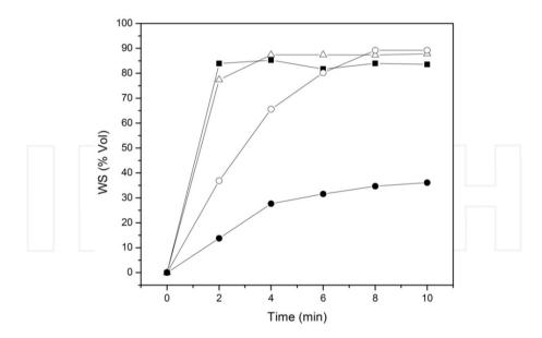
**Figure 7.** Kinetics of the separated water (WS) from the initial O/W emulsion treated under oil bath ( $\bullet$ ) and MW heating ( $\blacksquare$ ); and in the presence of a demulsifier (GlyC12, 1000 ppm) under oil bath ( $\circ$ ) and MW heating ( $\Delta$ ).
