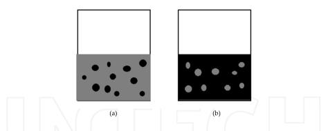
Figure 1. Representative scheme of two type of emulsions, oil-in-water (a) and water-in-oil (b) (oil in black, water in grey).
