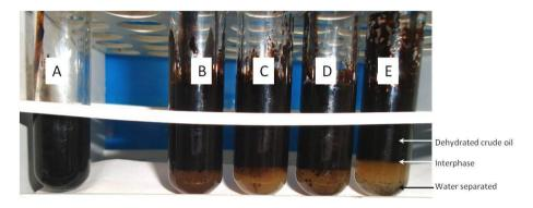
**Figure 8.** Photographs showing separated water (WS) from the initial O/W emulsion containing GlyC<sub>12</sub> (1000 ppm) at 50 W, 60°C. Initial O/W emulsion before MW irradiation (A), emulsion after MW irradiation during 2 (B), 4 (C), 8 (D), 10 minutes (E).
