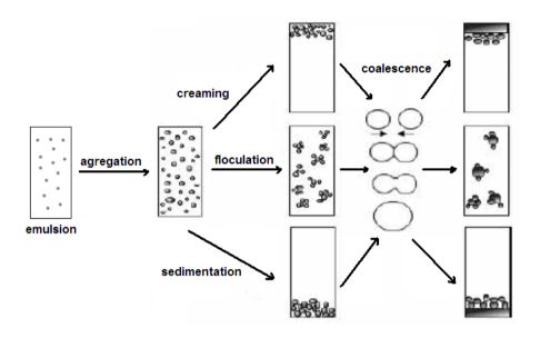
Figure 2. Scheme of emulsion breaking adapted from [4].
